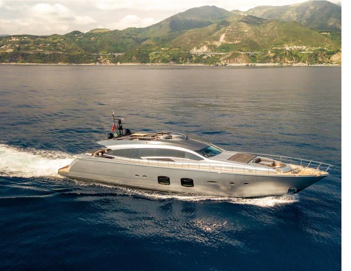
X-Trem II is a 33.23 m / 108' luxury motor yacht. She was built by Pershing in 2015 with exterior design by Fulvio de Simoni. With a beam of 6.7 m and a draft of 1.83 m, she has a GRP hull and GRP superstructure.
